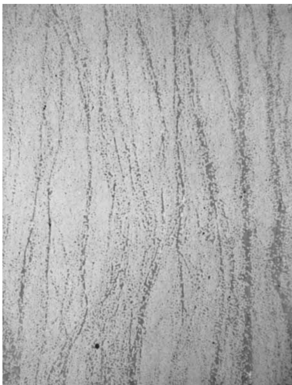
Fig. 1. Photomicrograph of PPQ system I/HMS graphite fiber; \times 50 .
